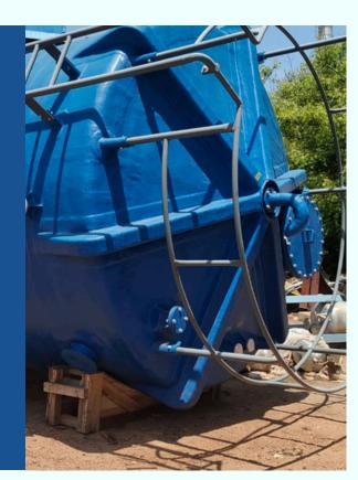
synthetic materials create corrosion barriers unique to composites. They design both the corrosion-resistant liner and structural wall, each with specific chemical and structural needs.
